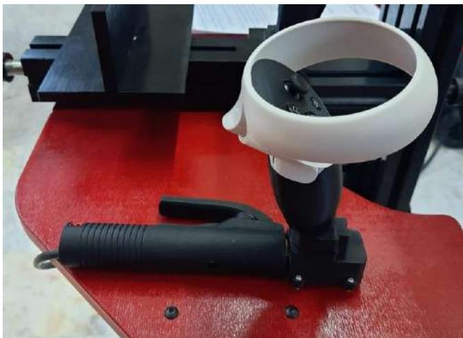
15. Mount the touch screen on the simulator device and connect the cables.
