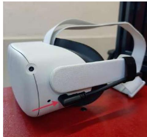
17. Plug the device into an electrical outlet 220 VAC 50-60 Hz and insert the other plug into the back of the device.
